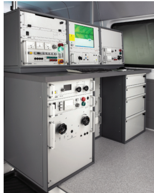
IRG 3000, integrated in the cable test van
